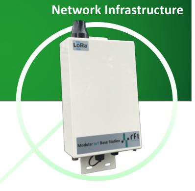
The function of the L-gateway is to forward received RF packets to an external server through a IP/UDP link. It also transmits RF packets that are sent by the external server. The L-gateway is standard equipped with one LoRa radio, a GPS receiver and an advanced 3G modem. Optionally it can be expanded with two additional radio's to turn the unit into a sectorized base station.
